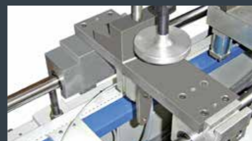
Pneumatic carriage between the two heads for the automatic shifting of the work piece when cutting short pieces. (TR2B I INT)
